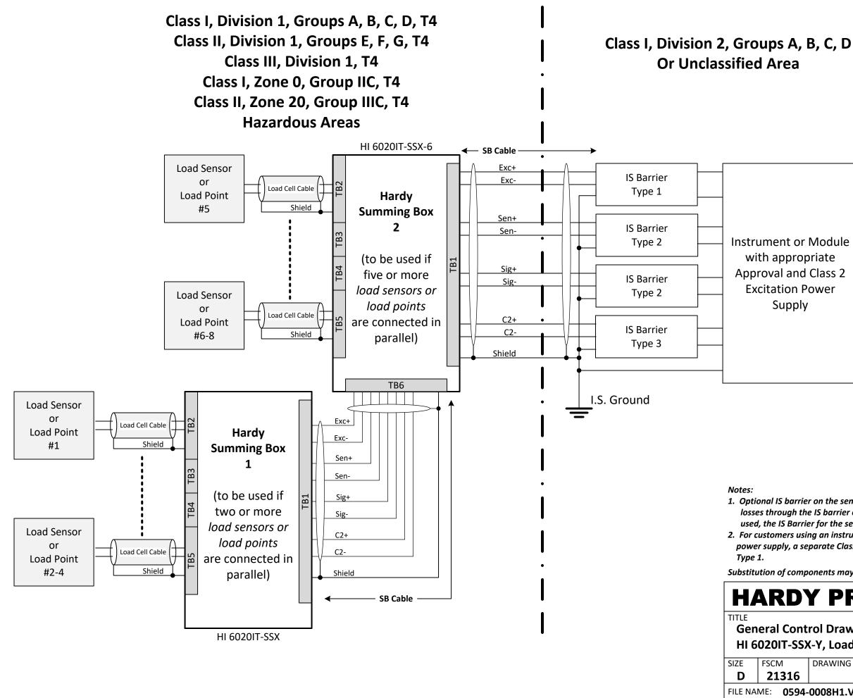
1. Optional IS barrier on the sense lines is used to automatically compensate for losses through the IS barrier on the excitation lines. If the sense lines are not used, the IS Barrier for the sense lines is not required 2. For customers using an instrument or module without a Class 2 rated excitation power supply, a separate Class 2 power supply can be used to power IS Barrier
